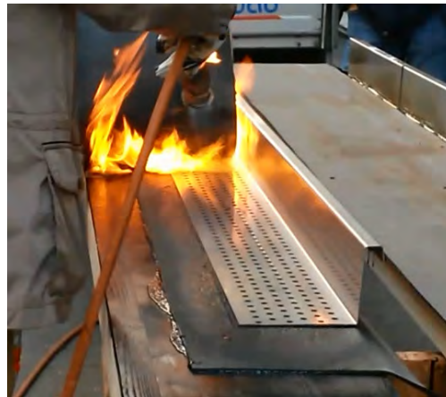
Figure 4.20. Test of welding the waterproof bitumen sheet on edge steel angle
